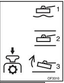
Pull lever backwards to LIFT (3) position to lift mower.
